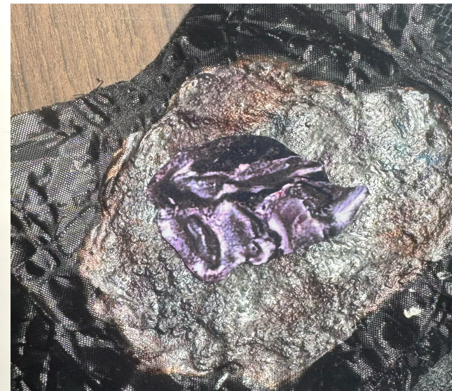
4. Completed Puff Binder Oil Spill Sample 1
